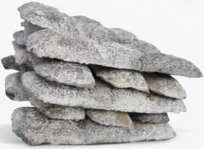
Ferronickel (FeNi) Material used to produce stainless steel.
