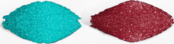
Nickel Sulfate (NiSo4) & Cobalt Sulfate (CoSo4) Material for precursor electric vehicle battery.
