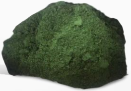
Mixed Hydroxide Precipitate (MHP) Intermediate nickel product produced by HPAL process.
